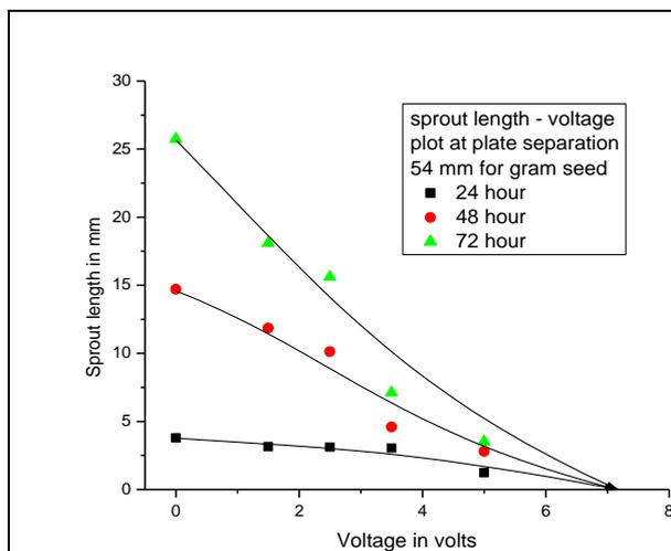
**Figure 4 (a) Variation of sprout length with voltage for different time of exposure to electrostatic field and voltage for germination at fixed plate separation 54 mm for gram seeds.**
