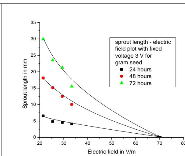
**Figure 5 (b) Variation of sprout lengths with electrostatic field for different time of germination at fixed voltage 3 V for gram seeds.**
