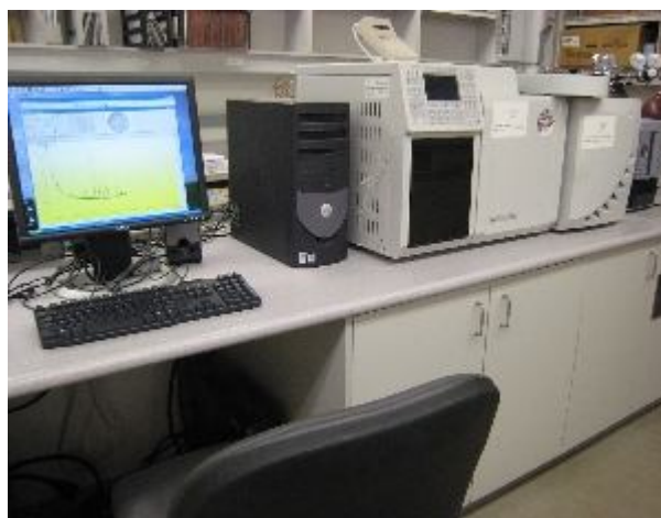
Fig 2. Laboratory equipment used for lipid, or fatty acid, analyses. The Gas Chromatograph separates the individual components of the residue sample. The instrument is equipped with two different detectors: a Flame Ionization Detector (FID) and a Mass Spectrometer (MS). Component identifications made with the FID are based on comparisons with standards. Components passing into the MS are identified with the computerized NIST Mass Spectral database, Photo courtesy of Mary Malainey.
